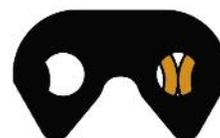
RPV and RP chain joint with "Crescent" shaped pins
