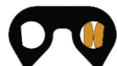
SC chain joint with "D" shaped pins
