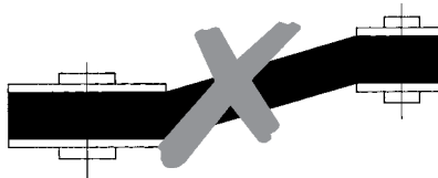
Axial misalignment of sheaves
