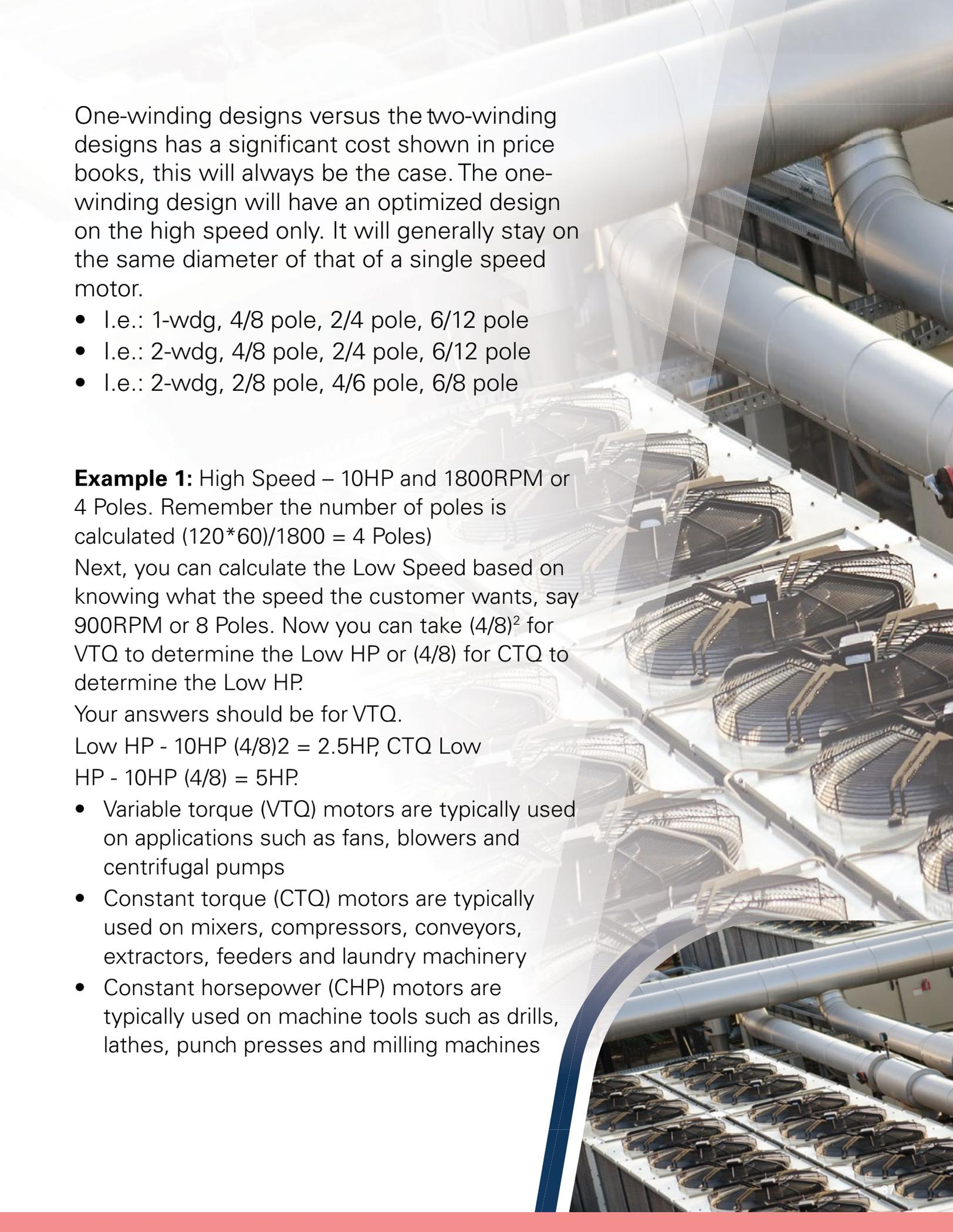
One-winding designs versus the two-winding designs has a significant cost shown in price books, this will always be the case. The one-winding design will have an optimized design on the high speed only. It will generally stay on the same diameter of that of a single speed motor.
