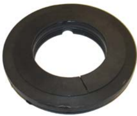
Failed Seal Resulting from Improper Fit
