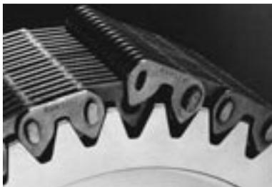
Symmetric chain lacing during connection
